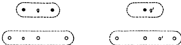
Fig. 24—Zero-sequence circuits formed by the 110 kv line (a), the 66 kv line (a'), the two ground wires (g), and the single ground wire (g').
