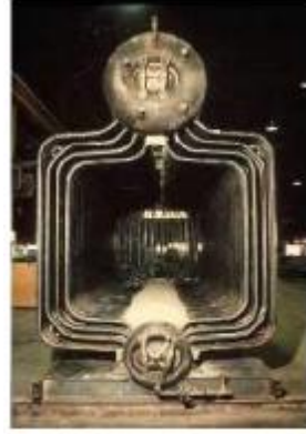
Watertube Boiler "O Type"
