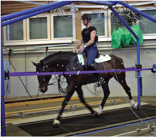
Fig 1.19 Horse and rider on the instrumented treadmill at the Zurich lab during the investigations into the effect of head and neck position on equine biomechanics. Both rider and horse are equipped with reflective markers; two ProReflex® cameras can be seen in the background. The small threads running to the hooves of the horses serve to determine the exact position of each limb, which is necessary input for the analysis of the force plate data.
