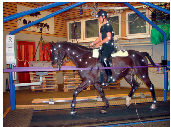
Fig 2.17 Horse being ridden on a treadmill instrumented for measurement of vertical ground reaction forces at University of Zurich, Switzerland. The hooves are attached by rubber bands to goniometers that triangulate the hoof positions.
