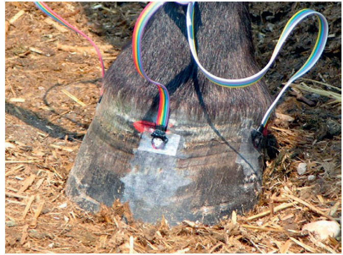
Fig 2.21 Strain gage attached to the hoof wall.
