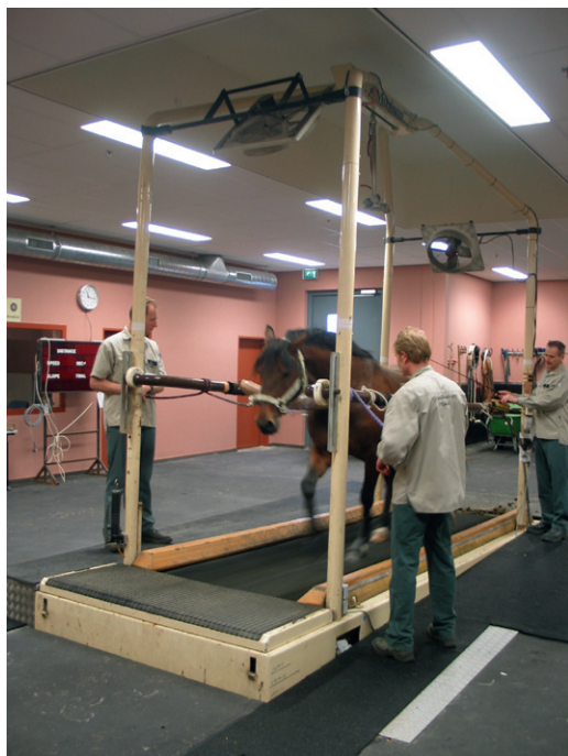
Fig 16.7 Treadmill used to induce early overtraining experimentally by de Graaf Roelfsema and co-workers.
