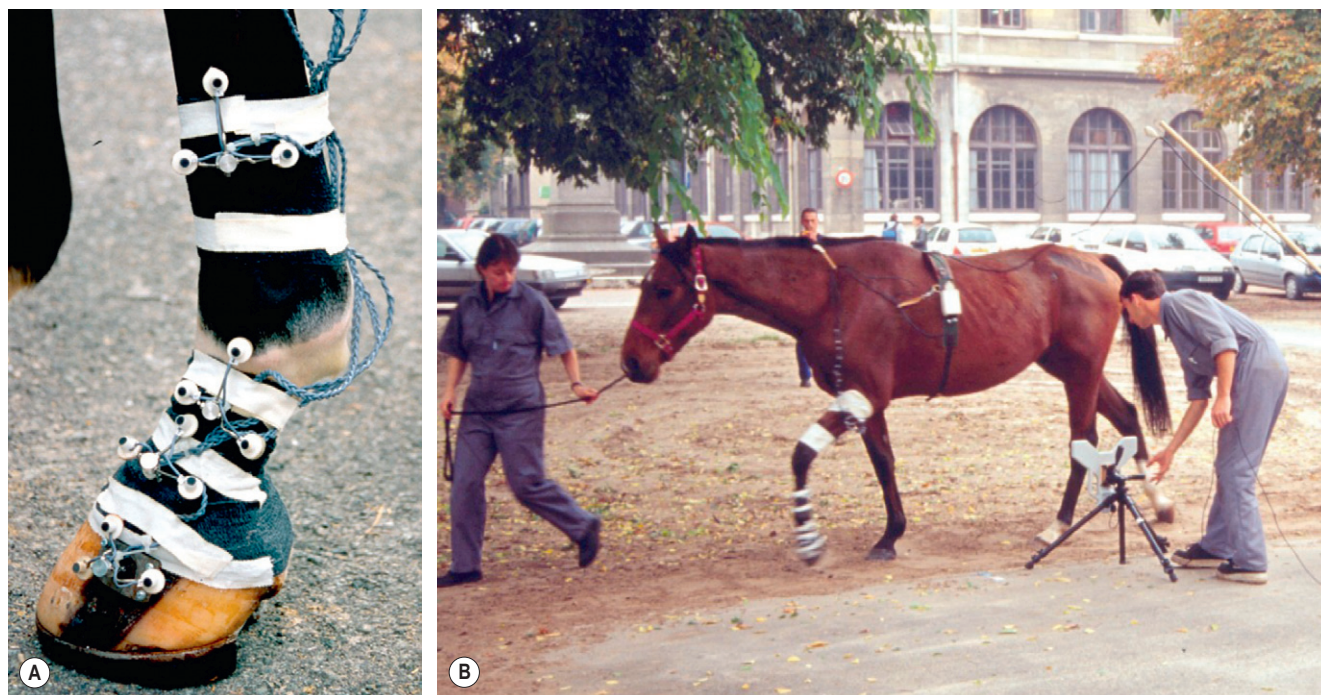
Fig 2.11 Zebris system in use at the National Veterinary School of Alfort, France. Triads of ultrasound microphones fixed rigidly to the limb segments (left) are located relative to a fixed system of three ultrasound transmitters as data are collected from a horse moving over ground (right).
