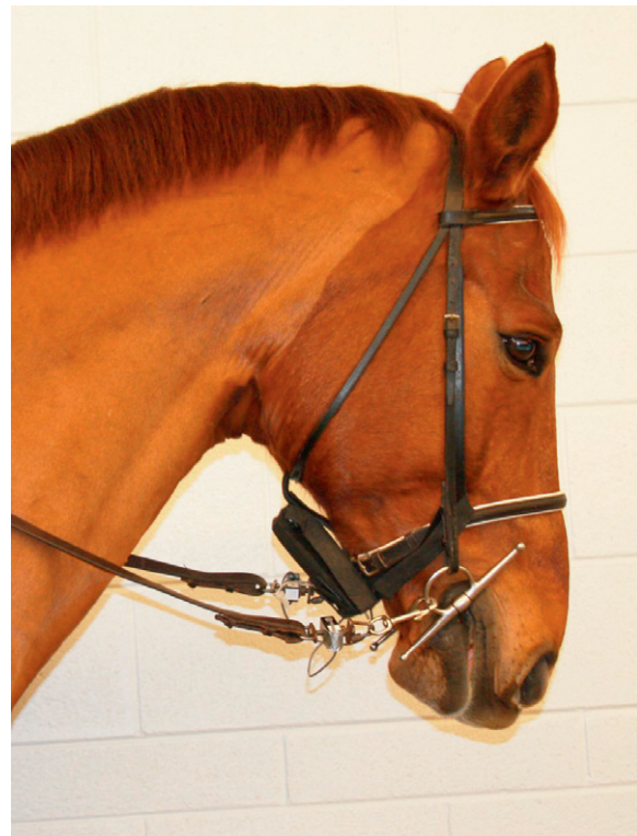
Fig 2.23 Telemetered system for measuring rein tension showing strain gages inserted between rein and bit with battery operated power source and transmitter-attached to the noseband underneath the horse's chin.
