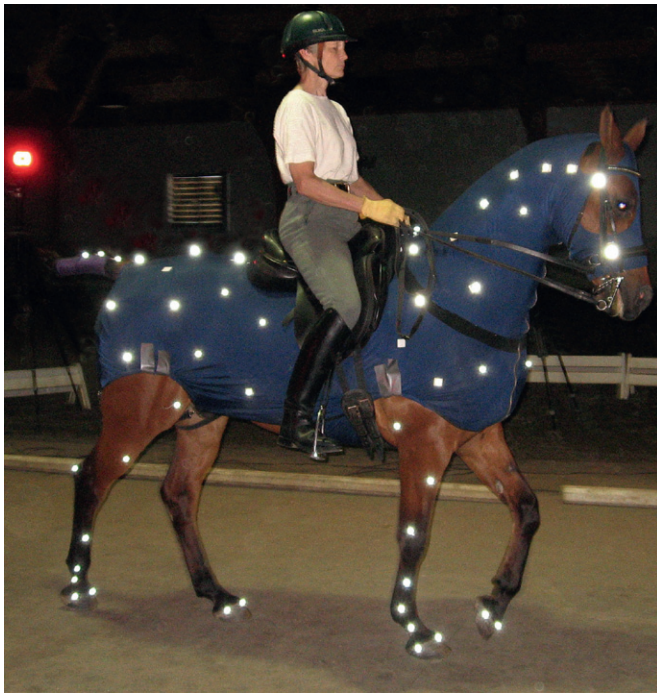
Fig 20.15 Dr. Hilary Clayton rides her horse MSU Magic J, who is wearing a blanket covered with predefined, anatomical markers, in front of an infrared motion capture system to develop an animation of the gaits of dressage horses.
