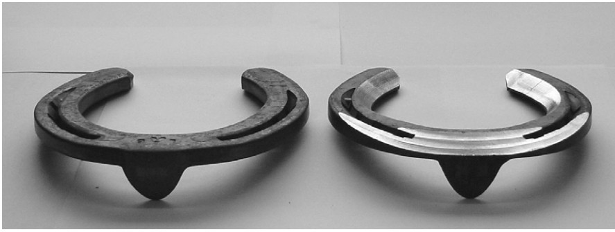
Fig 8.11 Shoes used to compare breakover. Left, a standard flat shoe (Mustad 22/10 LB); right and a shoe with a rolled toe (Mustad 22/10 equilibrium).
