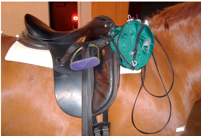
Fig 2.27 Pressure mat (Pliance, Novel GmbH, Munich, Germany) placed beneath saddle. Power source and transmitter are in the pack carried at the front of the saddle. The wires shown in loops on the horse's shoulder fit into the green bag during data collection.
