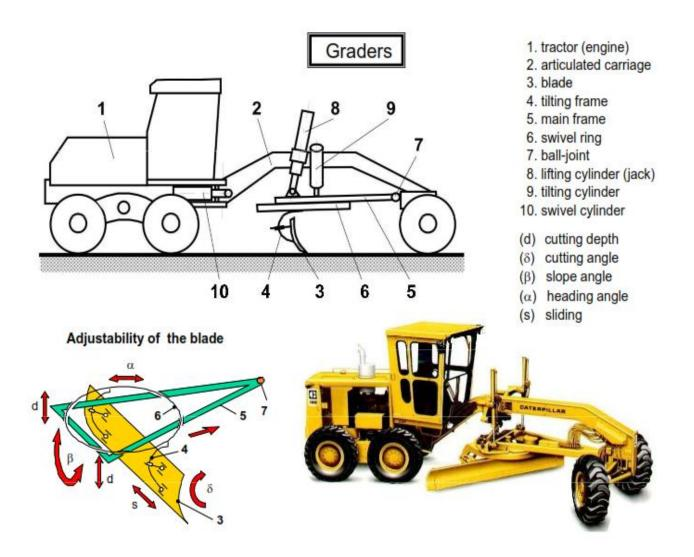
Figure - Principal parts of a motor grader.
