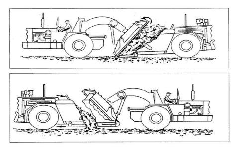
Figure- Typical Elevating Scraper
