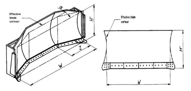
Figure 4 - Effective blade contour of semi-U- and U-blades
