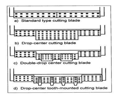
Figure – Cutting blade for Scraper
