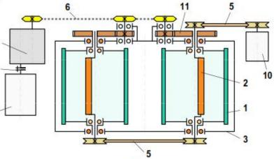
Double engine drive (both roller wheels are driven)
