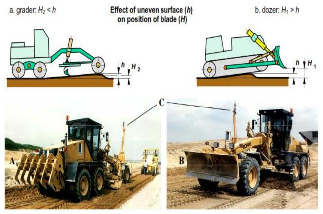
Laser controlled (C) grader equipped with ripper (A) and front blade (B) attachment
