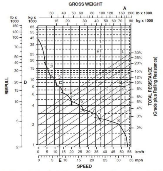
FIGURE Rimpull-speed-gradeability curves. (Source: Caterpillar Performance Handbook, 24th ed., 1993. Caterpillar, Peoria, IL.)
