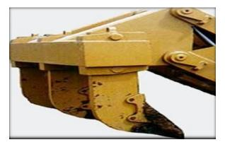
The ripper is the long claw-like device on the back of the bulldozer. Rippers can come as a single shank/giant ripper) or in groups of two or more (multi
