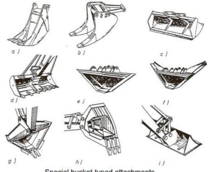
Special bucket-typed attachments a. drainer; b. ripper; c. canal maintainer; d. ripper-cleaner; e. profile bucket; f. extended cutter; g. ripper-profiler; h. ejector; i. tamper
