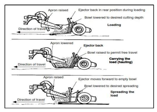
Figure - Functions of the Apron, Bowl, and Ejector
