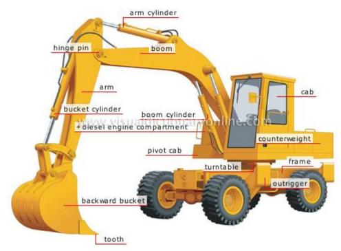
Modern, hydraulic excavators come in a wide variety of sizes. The smaller ones are called mini or compact excavators. For example, Caterpillar's smallest miniexcavator weighs 2,060 pounds (930 kg) and has 13 hp; their largest model is the largest excavator available (a record previously held by the Orenstein & Koppel RH400) the CAT 6090, it weighs in excess of 2,160,510 pounds (979,990 kg), has 4500 h.p and has a bucket size of around 52.0 m<sup>3</sup> depending on bucket fitted.
