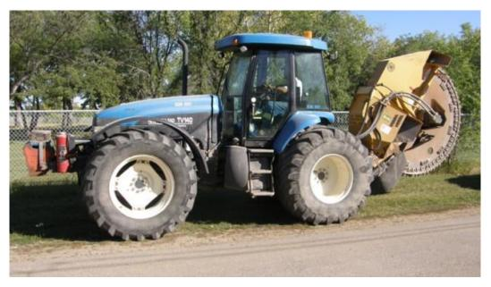
Wheel trencher attached to New Holland tractor
