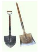
The wide mouth shovel is useful for picking up sand and other materials from hard surfaces and the pointed mouth shovel is used for excavation when large amounts of sand need to be removed.
