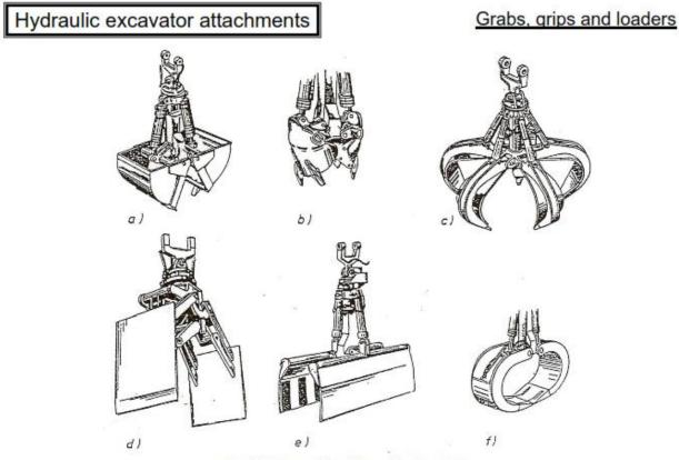
Grabbing and loading attachments a. clamshell; b. boring; c. fingered; d. bale grip; e. barrel/pipe grip; f. logger
