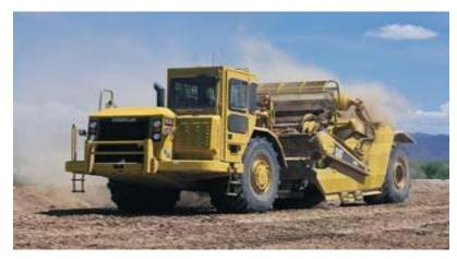
The ejector is a curved plate located at the back of the bucket. The ejector can be moved forwards to push material out of the bowl. Figure highlights the blade, apron, and ejector on a typical scraper bowl.
