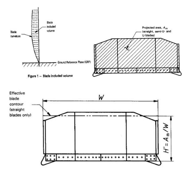
Figure 3 - Straight, semi-U-, U-blade dimensions
