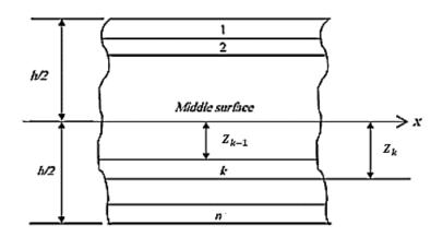
Figure 3.3 Geometry of an n-layered laminate
