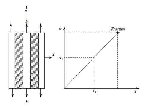
Figure (2.4) Unidirectional lamina loaded in the fiber-direction
