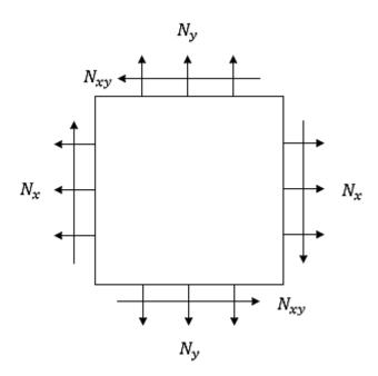
Figure (3.4) External forces acting on an element
