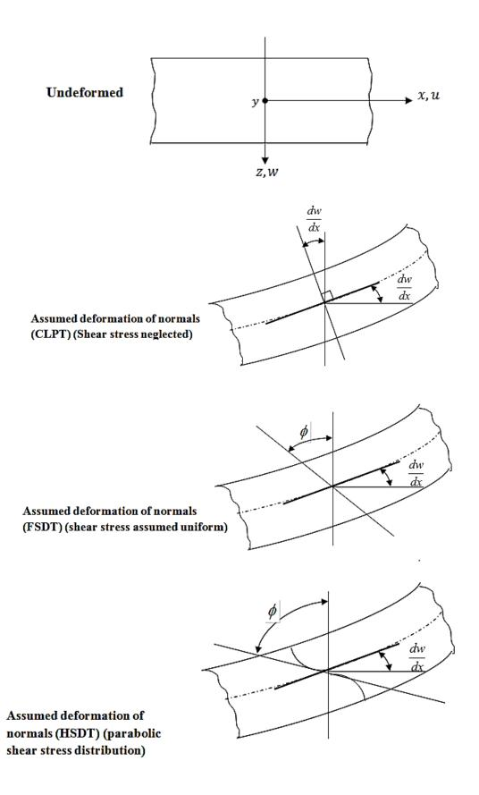
Figure (1.1) Assumed deformation of the transverse normal in various displacement base plate theories
