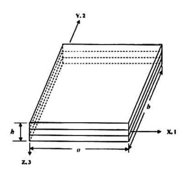
Figure 3.1 The geometry of a laminated composite plate
