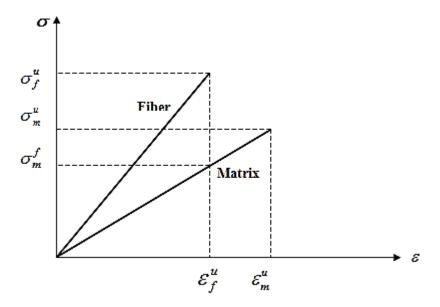
Figure (2.2) Stress-strain relationships for fiber and matrix
