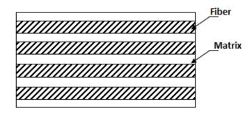
Figure (2.1) Structure of a fibrous composite
