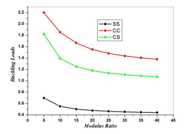
Figure (5.6) Effect of material anisotropy
