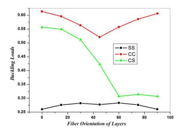
Figure (5.7) Effect of fiber orientation of layers,  $E_1/E_2=40$
