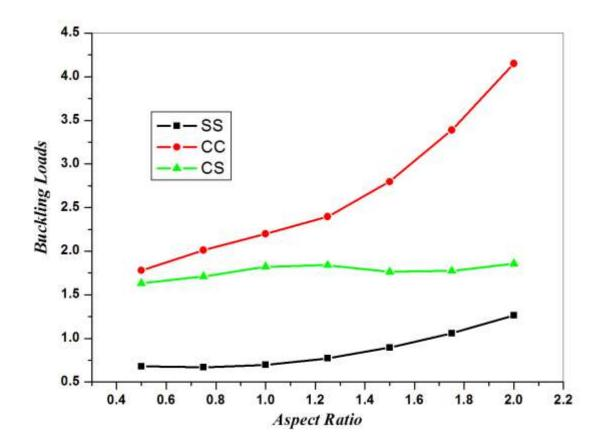
Figure (5.5) Effect of aspect ratio for different boundary conditions,  $E_1/E_2=5 \label{eq:energy}$
