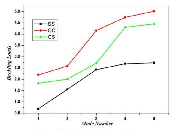
Figure (5.9) Effect of boundary conditions
