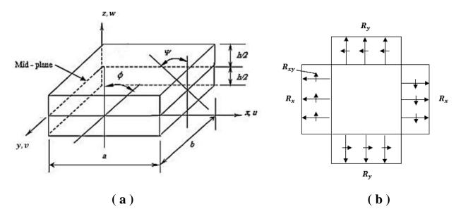
Figure 3.2 A plate showing dimensions and deformations
