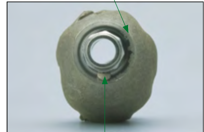
Casting beads and overflow of alloy on the 45 degree-shoulder.
