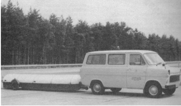
FIGURE 19.61 TRRL high speed road monitor (Source: Croney and Croney, 1998) (Copyright McGraww-Hill, New York, 1998, used by permission).
