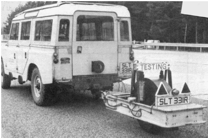
FIGURE 19.64 Bump integrator (Source: Croney and Croney, 1998) (Copyright McGraww-Hill, New York, 1998, used by permission).
