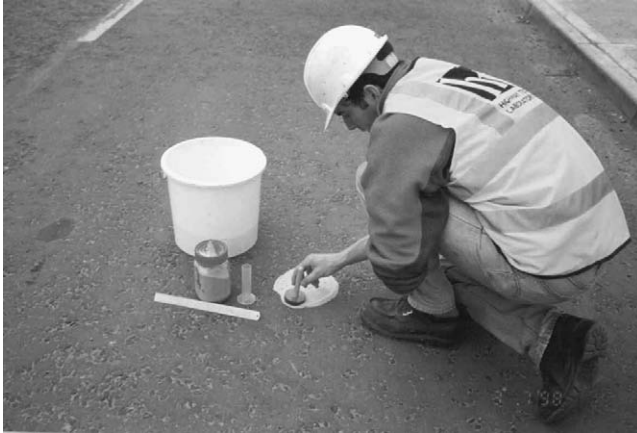
FIGURE 21.8 Volumetric patch test.
