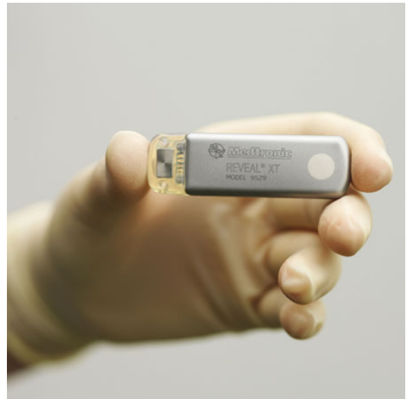
Figure 7.2. The Reveal XT (Medtronic Inc.) is an implantable device recording the cardiac rhythm for up to 3 years. Ongoing studies are evaluating these implantable loop recorders for the diagnosis of paroxysmal atrial fibrillation in patients with stroke.
