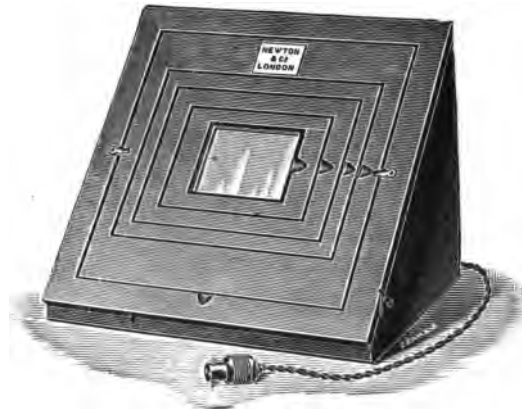
Fig. 51. Illuminating Desk for X-ray negatives.
