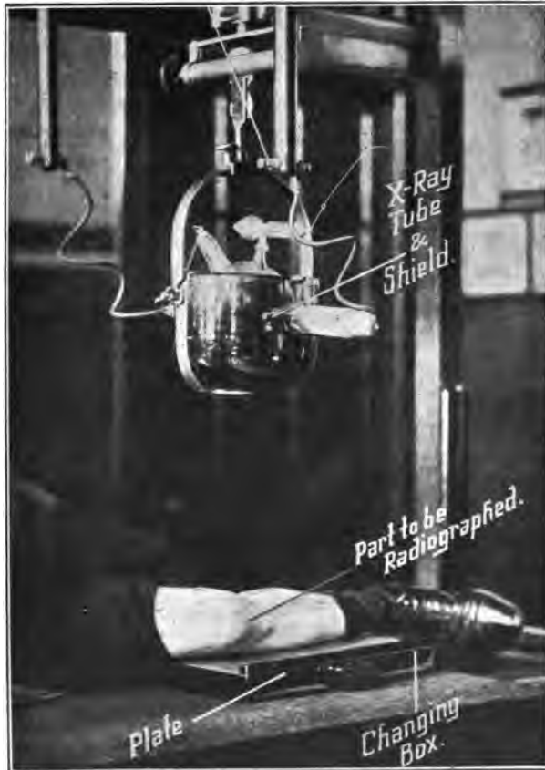
Fig. 50. Showing how to Radiograph a Knee.
