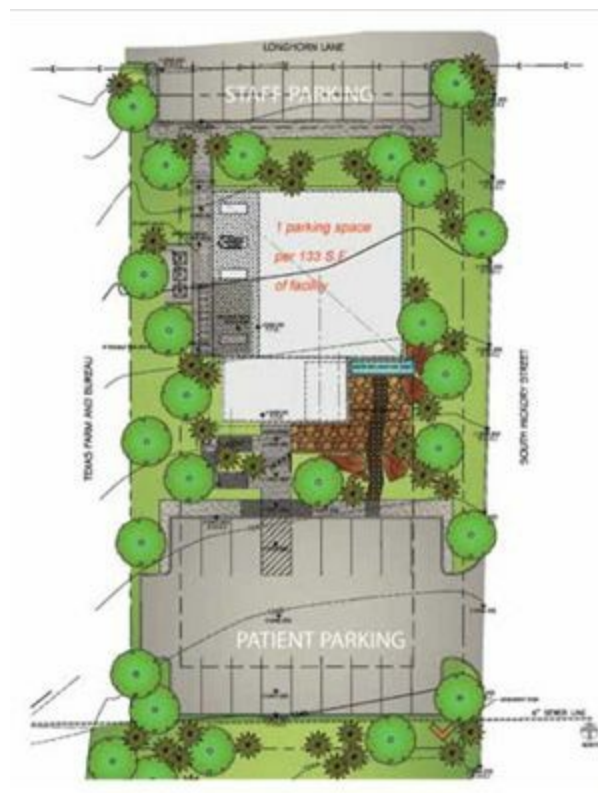
Site plan showing well configured and adequate parking for a dental facility
