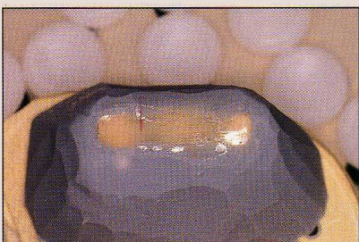
Fig 3-9g Polymerized Vectris Pontic within silicone matrix, prior to removal from the Vectris VS1 unit.
