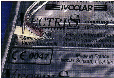
Fig 2-8 Pre-impregnated FRC strip being removed from its light-tight package.
