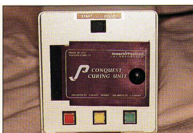
Fig 3-10p Conquest Curing Unit (Jeneric/Pentron), for the final application of heat under vacuum, used after the prosthesis is completed to maximize polymerization.
