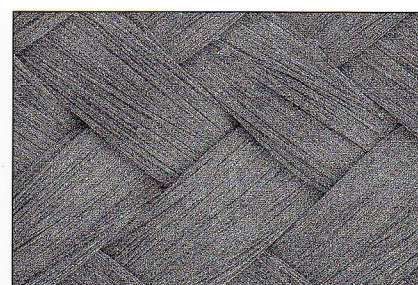
Fig 4-8 Scanning electron micrograph of GlasSpan Rope. (Original magnification x 100.)
