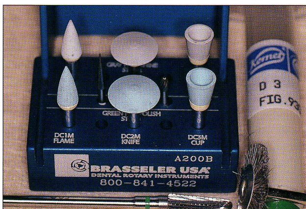
Fig 3-14 Instruments used to shape, finish, and polish the FRC prosthesis in the dental operator.
