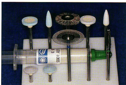
Fig 3-11 Instruments used to shape, finish, and polish the FRC prosthesis in the dental laboratory.
