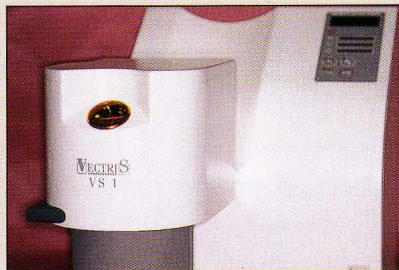
Fig 3-9e Vectris VS1 curing unit presses and light polymerizes the Vectris FRC material while under a vacuum.
