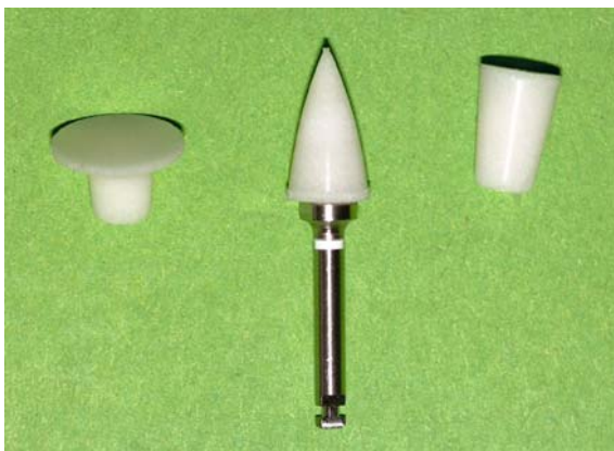
Fig. 5.5 Alumina- and silica-impregnated synthetic rubber points designed for polishing the resin composite
