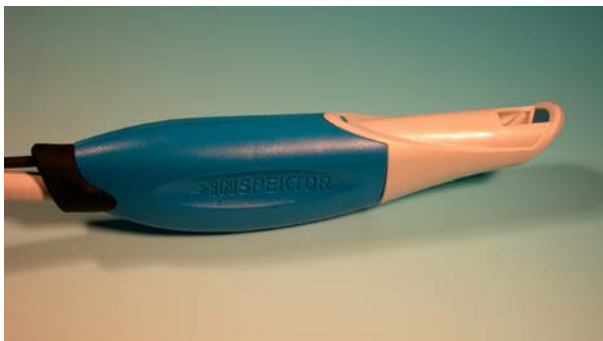
Fig. 1.6 The quantitative light-induced fluorescence system (QLF system, Inspektor Research Systems, Amsterdam, The Netherlands)
