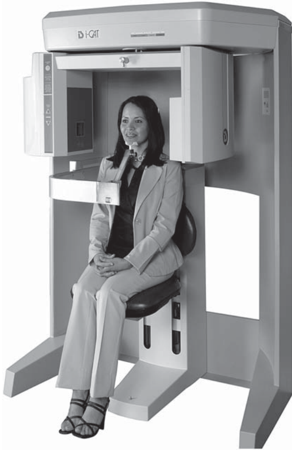
FIG. 14-1 Example of CBCT Unit. Imaging may be performed with the patient seated, supine, or standing. The patient's head is positioned and stabilized between the x-ray generator and detector by a head-holding apparatus. The detector may be a flat panel (this example) or image intensifier. During exposure the generator and detector rotate fully or partially around the patient's head. Scan time is as fast as 5 seconds. Most CBCT units have a small "footprint" enabling in-office placement. (Courtesy Imaging Sciences International, Hatfield, Pa.)
