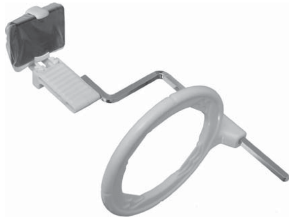
FIG. 3-6 XCP film-holding instrument. The aiming ring aligns a circular aiming cylinder from an x-ray machine with the sensor to assure that the image plane is perpendicular to the central ray and in the middle of the beam. Note notches to align rectangularly collimated aiming devices such as shown in Figures 3-5 or 3-7. Sensor is in plastic bag to prevent contamination from saliva. (Courtesy Dentsply Rinn, http://www.rinn corp.com/ .)
