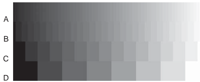
FIG. 7-8 Contrast resolution. Examples of gray-scale ramps representing distinct gray levels from black to white. Bit depth controls the number of possible gray levels in the image. The actual number of distinct gray levels that are displayed is dependent on the output device and image processing. The perceived number of gray levels is influenced by viewing conditions and the visual acuity of the observer. A , 6 bits/pixel—64 gray levels. B , 5 bits/pixel—32 gray levels. C , 4 bits/pixel—16 gray levels. D , 3 bits/pixel—8 gray levels.
