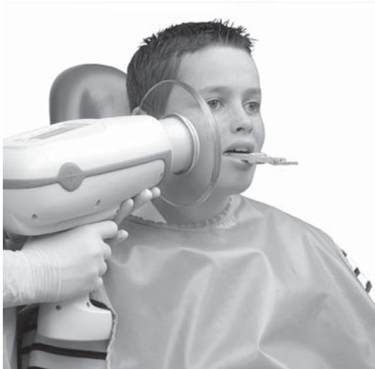
FIG. 9-11 Handheld x-ray machine useful for patients in remote situations. Operator dose is reduced by internal shielding and shield on aiming cylinder to reduce backscatter. (Courtesy Aribex, Inc.)
