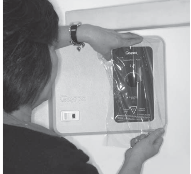
FIG. 8-7 Plastic wrap covers parts of console that are touched during the radiographic examination.
