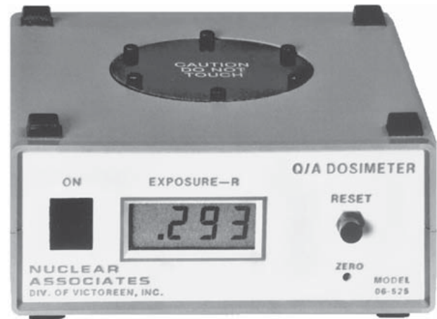
FIG. 8-5 Device for measuring exposure output of an x-ray machine. The aiming cylinder of the x-ray machine is positioned on the center of the top and an exposure made. The display on the front gives the output in roentgens.
