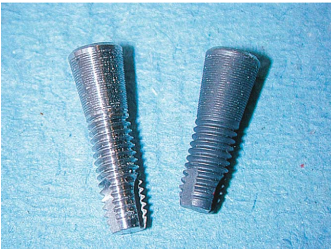
Fig. 12.76 Examples of a commercially available implant with screw thread. One surface is machined titanium (left) and the other has been titanium-blasted (right).
