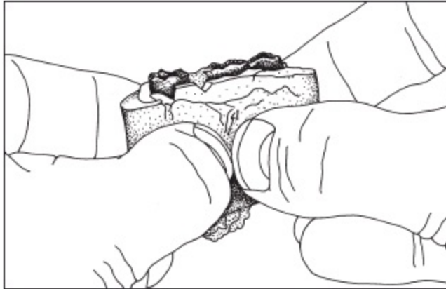
Fig 26-28 The investment is removed after placing it in water.
