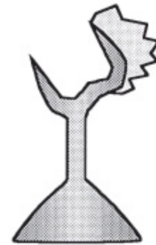
Fins— Dropped ring, rapid heating of wet or unhardened mold, liner flush with end of ring. Excessive casting force.
