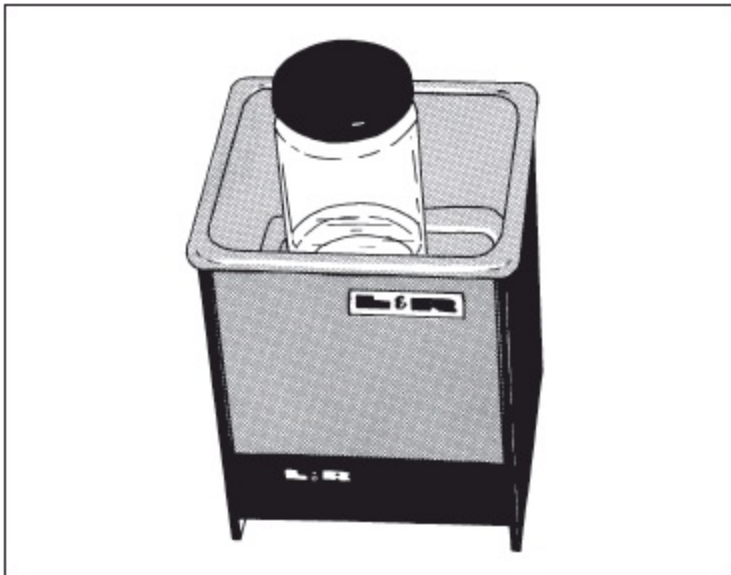
Fig 23-51 The veneer is placed on a piece of gauze in a jar, and the jar is placed into an ultrasonic cleaner.
