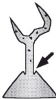
Random porosity— Dirt in wax pattern. Loose particles of investment from sharp edges (arrow).
