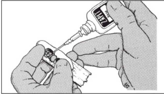
Fig 26-58 Zapit cyanoacrylate liquid resin is squeezed into the joint.
