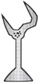
Shrink-spot porosity— Sprue attachment too bulky. Sprue too long or thin. Button too small.
