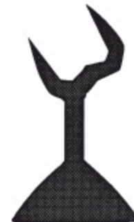
Black, rough casting— Breakdown of investment from excessive heat.
