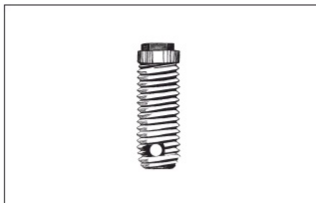
Fig 27-6 Endosseous implants were first introduced as a threaded root form with an external hex.
