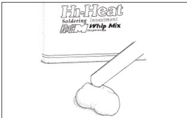
Fig 26-64 Crowns are filled with soldering investment.
