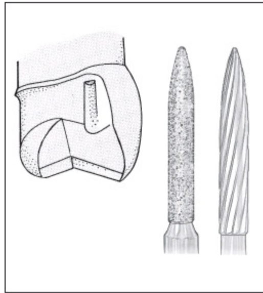
Fig 11-11 Proximal flares: flame diamond and bur.
