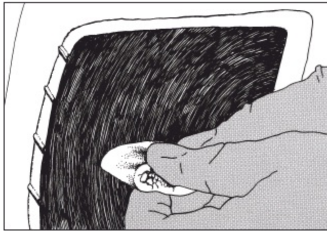
Fig 26-18 The cast trimmer is used to remove excess height from the block of investment.
