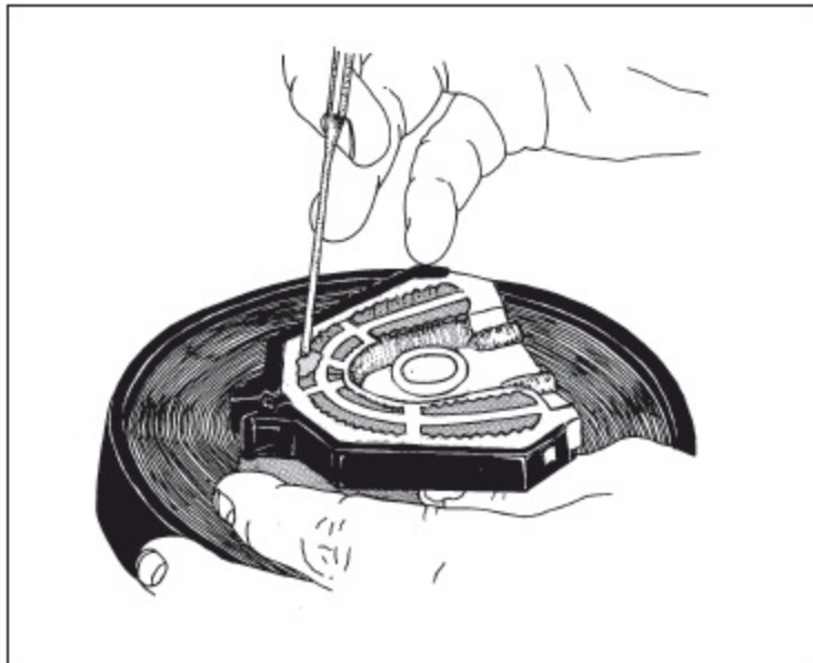
Fig 23-41 Refractory material is poured through openings in the underside of the die tray.
