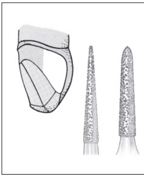
Fig 11-37 Proximal axial reduction: medium-grit long needle and coarse-grit tapered torpedo diamonds.
