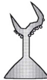
Nodules on underside only— Prolonged vibration after pouring.
