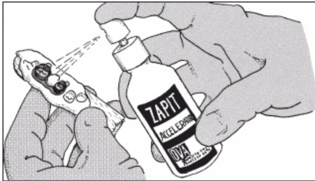
Fig 26-59 Zapit accelerator is sprayed into the joint.
