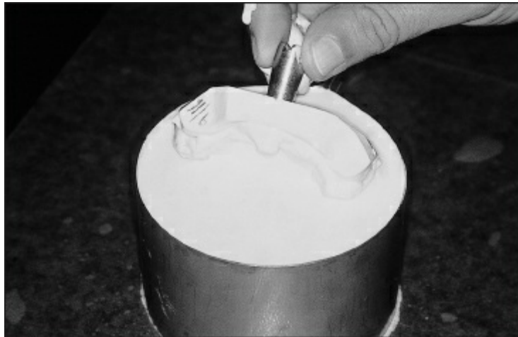
Fig 11-39 The refractory cast is carefully placed into freshly mixed investment in the mold former.
