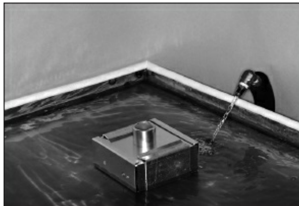
Fig 9-24 Reversible hydrocolloid-filled duplicating flask placed in water bath for 45 minutes to solidify liquid duplicating material.
