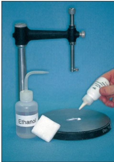
Fig 7-75 The platform of the surveyor and the base of the surveying table should be cleaned using an acetone- or alcohol-soaked gauze pad. A small amount of polymethyl methacrylate powder may be placed on the platform to minimize friction. The spherical particles of the polymethyl methacrylate serve as tiny ball bearings and thereby facilitate movement of the surveying table across the platform.
