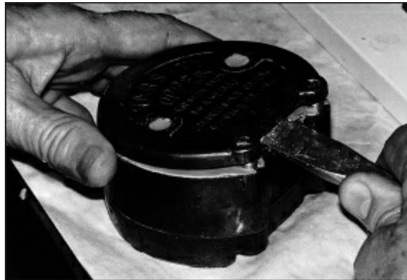
Fig 15-85 The lid of the flask is removed by prying with a chisel.
