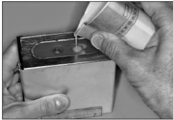
Fig 9-28 Clear autopolymerizing acrylic resin, mixed according to manufacturer instructions, is poured into the mold in the reassembled duplicating flask. Note that material is visible in vent channel, indicating the mold is filled.
