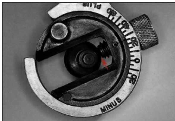
Fig 15-30 This condylar element is fully seated in its housing. No space is evident between the condylar element and the posterior stop ( arrow ).
