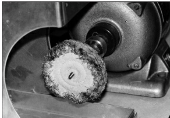
Fig 15-113 The prepared cloth wheel has a smooth, soft surface.
