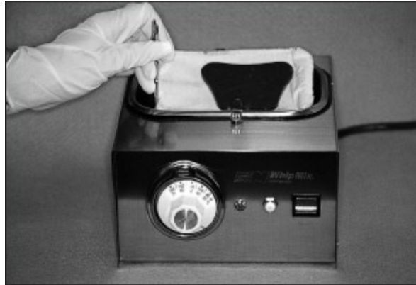
Fig 5-24 Modeling plastic is softened in a water bath at 60°C (140°F).
