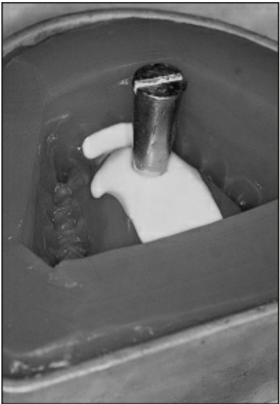
Fig 11-26 Refractory material is carefully flowed into the mold.
