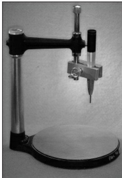
Fig 10-50 A dental surveyor may be used as a milling device. A handpiece holder is attached to the vertical arm of the surveyor. A straight handpiece is then secured parallel to the vertical arm of the surveyor in the handpiece holder.
