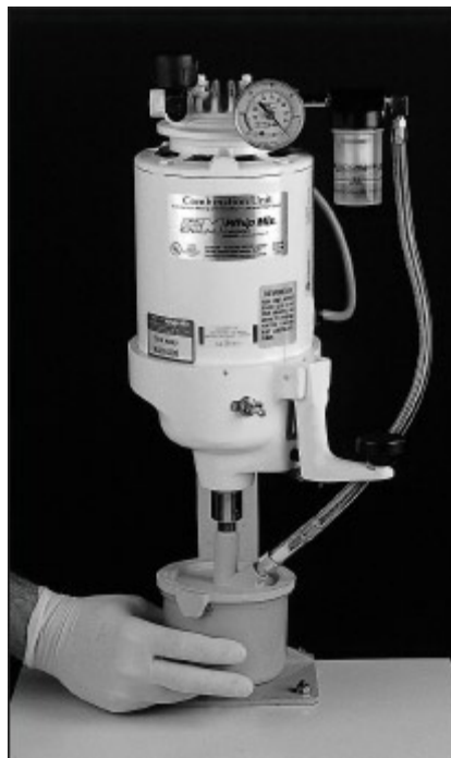
Fig 5-59 Dental stone is mechanically spatulated under vacuum for 15 to 20 seconds.
