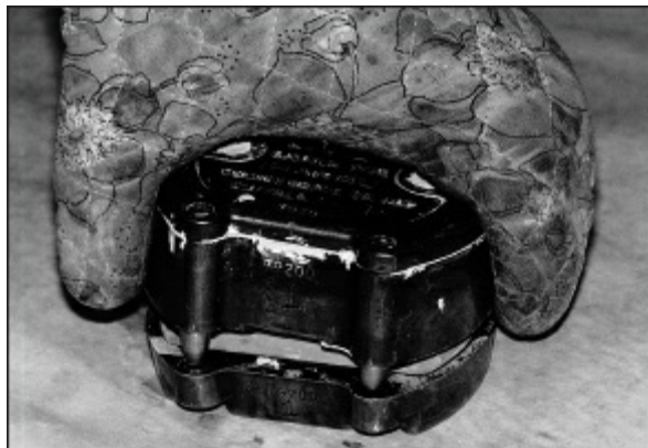
Fig 15-63 The upper portion of the flask is lifted as vertically as possible to avoid fracturing the investment layers.
