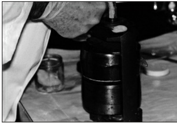
Fig 15-79 The flask is placed into a flask carrier and pressure is applied. The resin is given sufficient time to flow.
