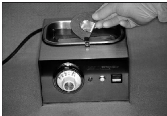
Fig 6-49 The metal-impregnated wax is softened in a water bath maintained at 43°C (110°F).
