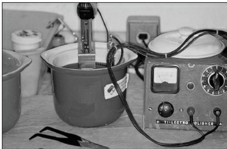
Fig 11-50 The Ti-Lectro Polisher produces a satin-like surface.
