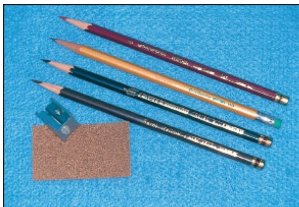
Fig 7-78 Red, black, blue, and brown pencils are used for survey and design procedures. A pencil sharpener and sandpaper should be available to ensure that lines are crisp and well defined.
