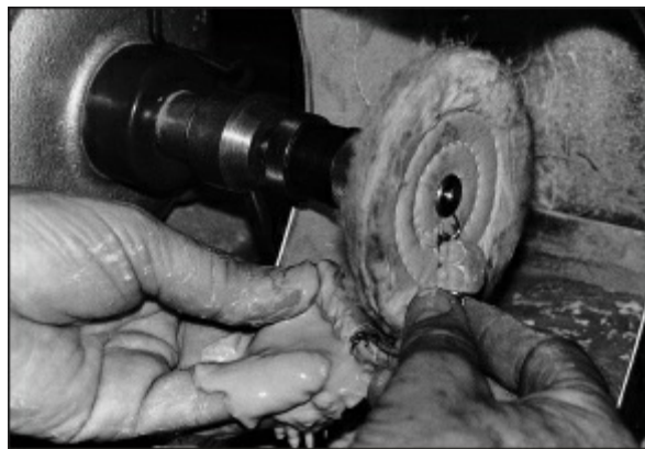
Fig 15-110 Acrylic resin borders are smoothed using flour of pumice on a wet cloth wheel.
