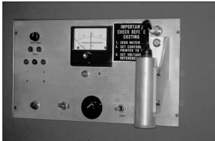
Fig 11-42 An electronic sensor measures the temperature of the molten metal. When the chosen alloy reaches the appropriate temperature, this sensor activates the casting process.
