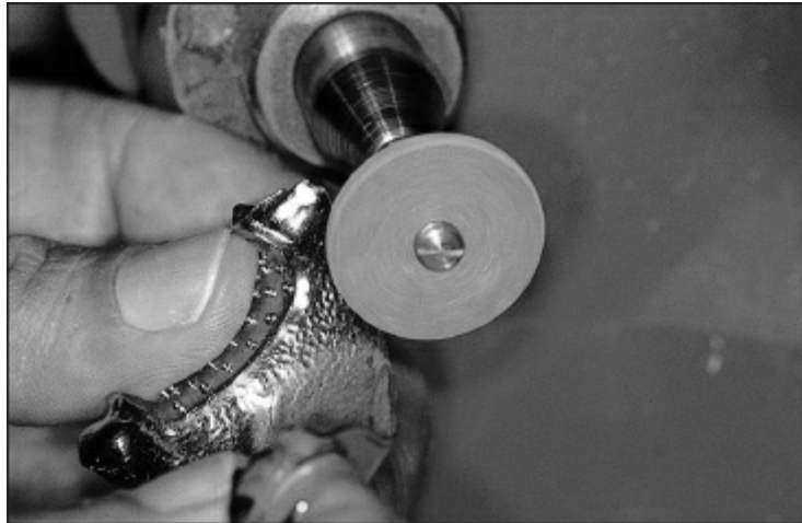
Fig 11-49 Finishing procedures are accomplished on a high-speed lathe.
