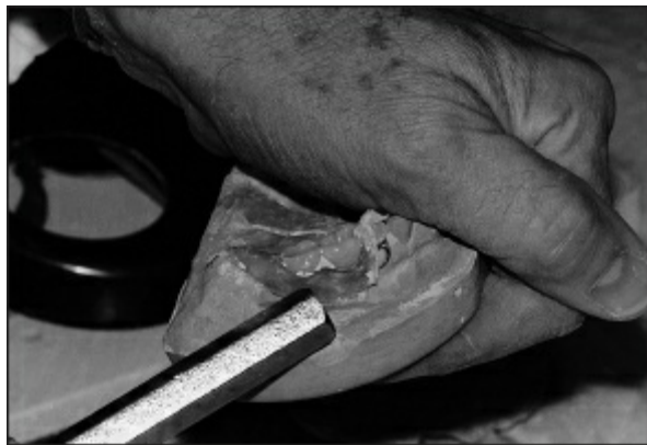
Fig 15-96 The first investment layer is removed by tapping with a chisel.
