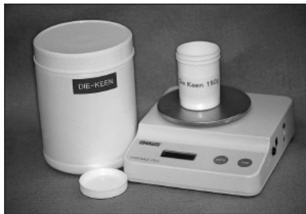
Fig 5-58 Gypsum products should be proportioned by weight and stored in properly labeled, moisture-proof containers.
