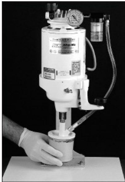
Fig 5-39 The mixing bowl is properly assembled, the vacuum tubing is attached, and the alginate impression material is spatulated for 15 seconds.
