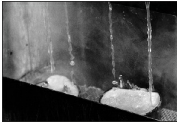
Fig 15-65 The remainder of the wax is flushed from the mold with boiling supernatant dental slurry.
