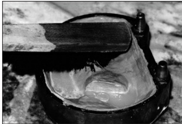
Fig 15-66 A soft brush and mild detergent are used to clean wax residue from the mold.
