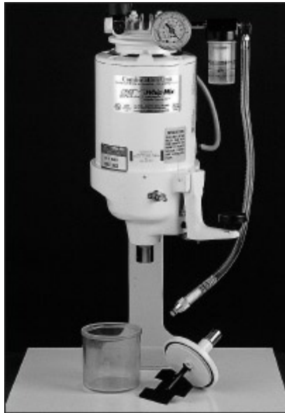
Fig 5-37 Vacuum spatulation is performed using a specially designed mixing apparatus consisting of a rotary mixing device, a vacuum pump, and the associated mixing bowl.
