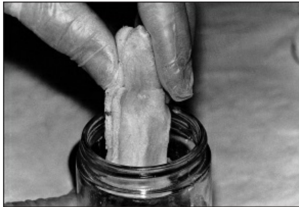
Fig 15-75 When the consistency of the resin is correct, it will separate cleanly from the mixing jar. Notice that the operator is wearing plastic gloves.
