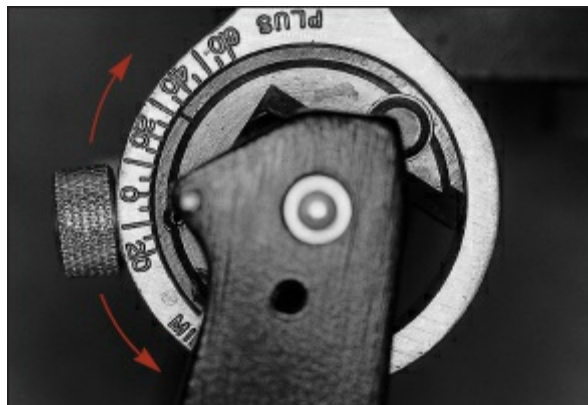
Fig 6-79 Each condylar inclination mechanism is rotated ( arrows ) to determine the appropriate setting.
