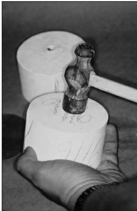
Fig 11-45 The framework is recovered by lightly tapping the investment with a hammer.
