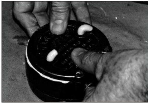
Fig 15-62 The fourth investment layer is used to fill the remainder of the flask. The lid of the flask is pressed into place while the investing stone is still soft.
