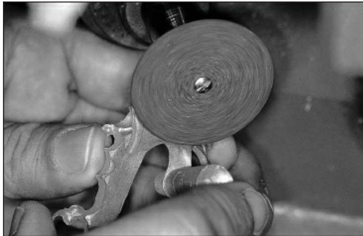
Fig 11-47 The sprue lead is removed using an abrasive disk.
