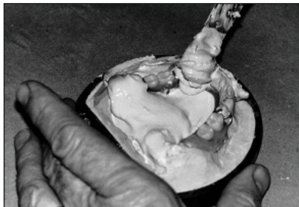
Fig 15-52 The second investment layer is added.
