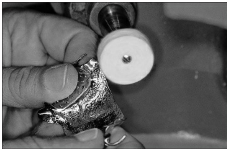
Fig 11-54 The framework is polished using felt wheels and fine-grit polishing agents.
