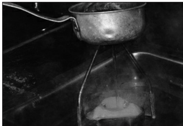
Fig 15-67 Residual detergent is removed by flushing the mold with clean boiling water.
