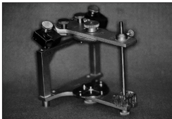
Fig 14-12 The Whip-Mix articulator (Whip-Mix) is a semiadjustable instrument.
