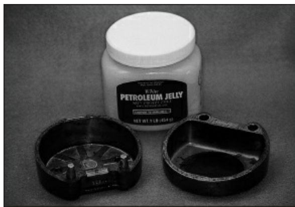
Fig 15-44 A thin film of petroleum jelly is applied to the surfaces of denture flasks to prevent oxidation of the metal.
