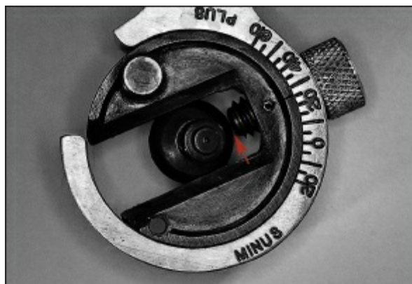
Fig 15-31 This condylar element is not fully seated in its housing. Space is evident between the condylar element and the posterior stop ( arrow ).
