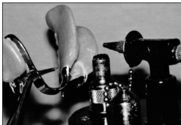
Fig 18-11 Denture bases are burned away from the underlying framework before the
