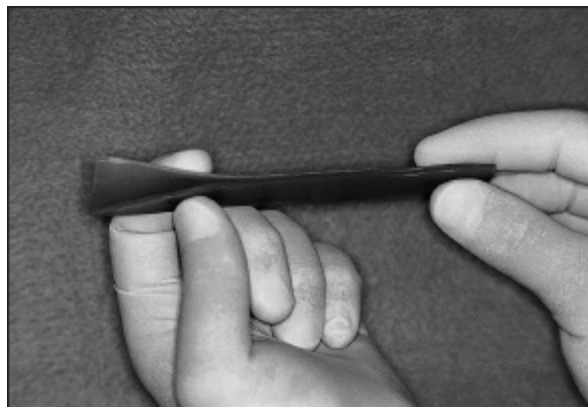
Fig 6-40 When the wax is pliable, it is folded lengthwise.
