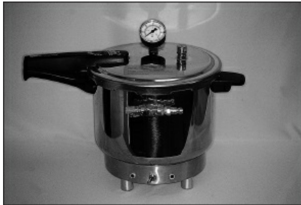
Fig 18-19 The assembly is placed in a heated pressure pot to complete the polymerization cycle.
