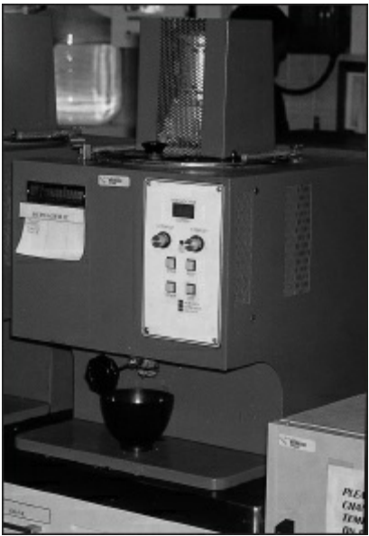
Fig 11-25 An automated duplicating machine is used in the preparation and storage of reversible hydrocolloid impression material.
