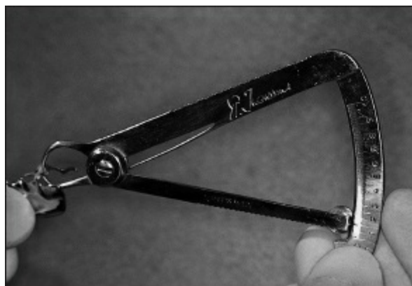
Fig 17-16 A metal thickness gauge is used to evaluate the thickness of removable partial denture components. Rests and clasps must be at least 1 mm thick.
