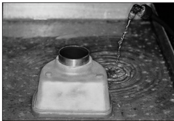
Fig 11-23 The base of the flask rests in a container of cool, running water.
