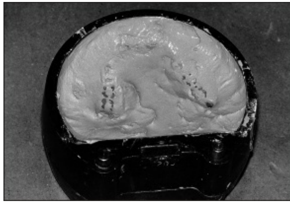
Fig 15-59 The surface of the third layer is left slightly rough to hold the fourth investment layer in position.
