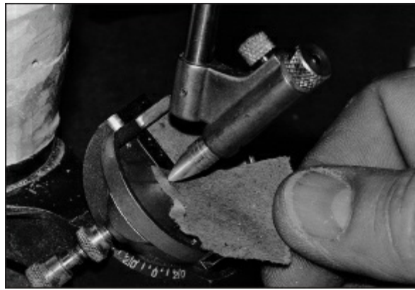
Fig 15-102 Occlusal correction is continued until the incisal pin contacts the incisal table.
