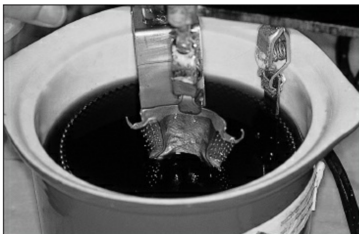
Fig 11-50 The Ti-Lectro Polisher produces a satin-like surface.
