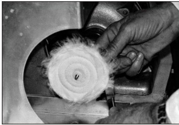
Fig 15-111 A new cloth wheel is prepared for use by running the wheel against the dull blade of a laboratory spatula. This loosens the fibers of the wheel.
