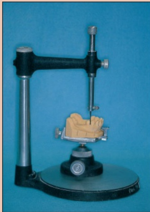
Fig 7-95 The mandibular cast is placed on a surveying table and locked in position. The practitioner should ensure that the occlusal plane is oriented parallel to the bench top.
