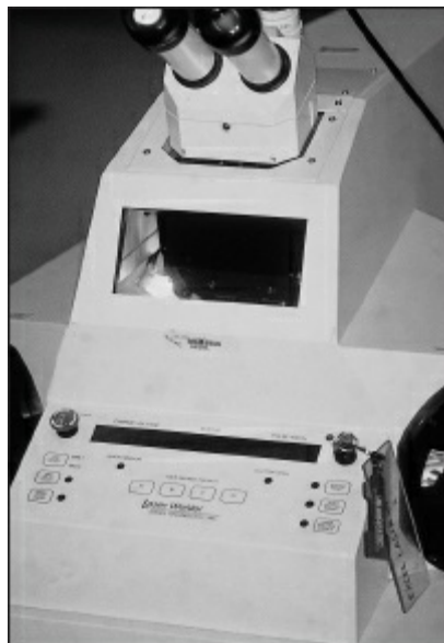
Fig 11-63 A laser welder can be used to join components of a removable partial denture.
