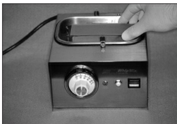
Fig 6-39 A wax strip of appropriate dimensions is placed in a water bath maintained at 60°C (140°F).
