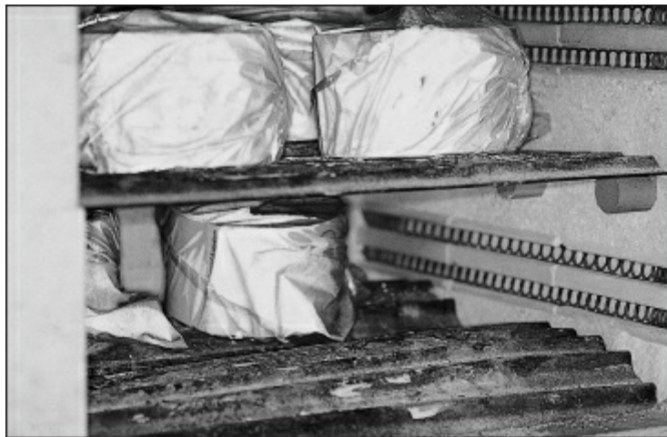
Fig 11-40 Plastic bags containing molds are placed in a burnout furnace.
