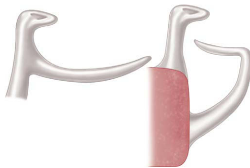
FIGURE 7-42 Length of the tapered cast retentive clasp arm is measured along the center portion of the arm until it joins the clasp body (circumferential) or becomes part of the denture base or is embedded in the base (bar-type clasp).
