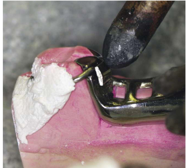
FIGURE 18-21 Wrought wire can be soldered to cast frameworks as an alternative method to incorporation in the wax pattern and casting procedure. Electric soldering is a common method for soldering and does not require heating of the entire framework. Following preparation of the minor connector where the wire will be soldered, an 18-gauge, round, wrought-wire clasp is carefully adapted and then is secured to the framework and the duplicate stone cast with the use of refractory investment. In this situation, a distolingual molar undercut will be used bilaterally for retention. The flux is placed at the proximal plate, followed by placement of sufficient solder, and the electric heat element tip is placed into contact with the solder while the frame is grounded at another location.
