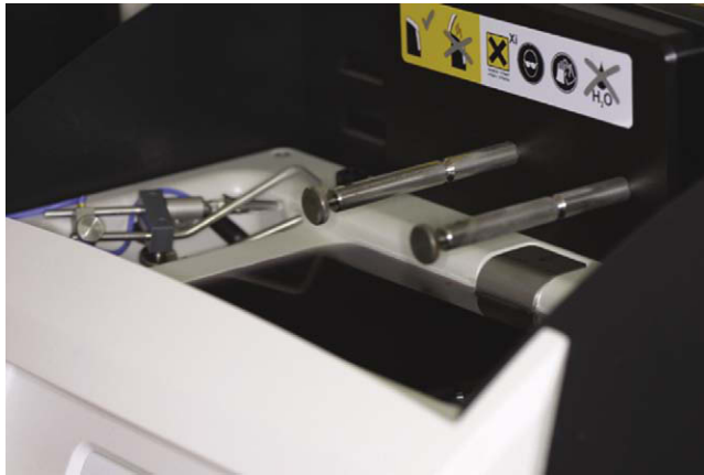
FIGURE 18-32 Electropolish unit used for the final surface polish of frameworks in a heated polishing liquid.
