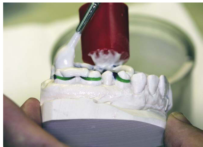
FIGURE 18-26 Applying the investment with a soft moistened brush to ensure complete adaptation of the investment. This will help reduce the number of bubbles and will make for a smoother cast surface.
