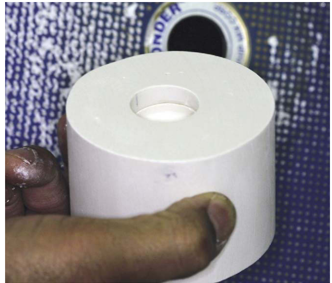
FIGURE 18-27 Investment mold has been trimmed to prepare the sprue end for burnout and subsequent complete adaptation to the casting machine.
