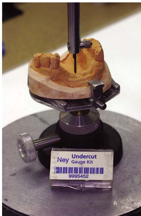
FIGURE 7-36 Essential parts of a dental surveyor (Ney Parallelometer, Dentsply Ceramco, Burlington, NJ), showing the vertical spindle in relation to an adjustable table.
