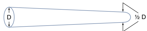
FIGURE 12-26 Round, 18-gauge wrought wire for the retentive component of the direct retainer assembly (clasp) is uniformly tapered to 0.8 mm from its full diameter to its terminus. Tapering should precede contouring of the wire for the retainer arm.
