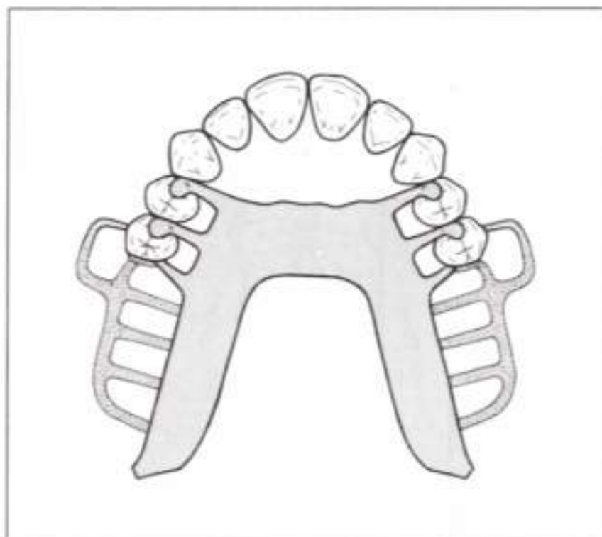
Fig. 14.1-11 A U-shaped major connector may be selected if (1) there is an inoperable torus which extends to within 6 to 8 mm of the vibrating line, or (2) the patient is unable to tolerate an anterior-posterior palatal strap. The U-shaped connector is the last choice because it often lacks rigidity and covers considerable tissue in an area prone to inflammatory papillary hyperplasia.
