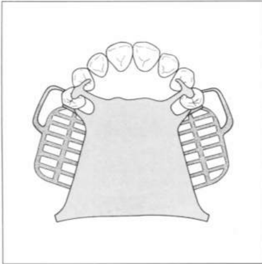
Fig. 4-18 A palatal plate major connector.
