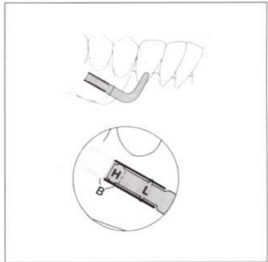
Fig. 6-55 An Oddo hinge in combination with an I-bar on a mandibular canine. Hinge (H); latch (L); retentive box or housing (B).
