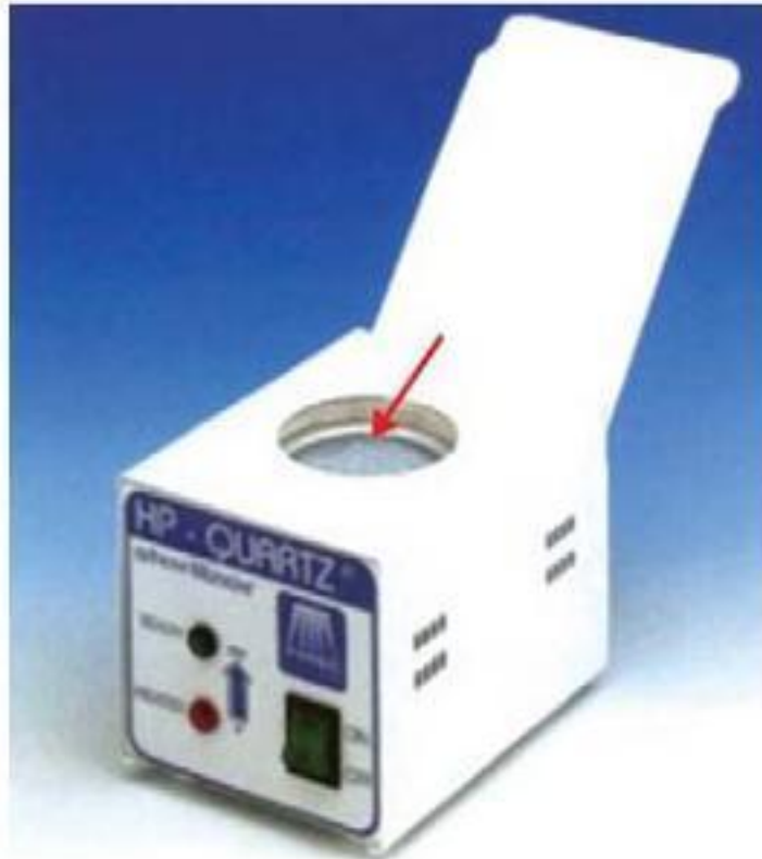
Fig. 2.1: Glass bead sterilizers (Arrow shows cup of glass bead)
