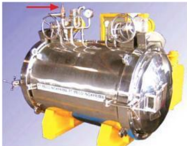
Fig. 2.2: Modern autoclave machine (Arrow shows safety valve)
