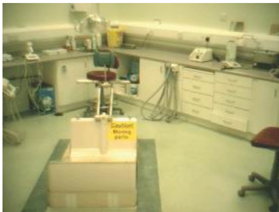
Fig. 17.22 A customized floor insert to accommodate a patient's wheelchair (courtesy of Dr Alistair Boles, National Rehabilitation Hospital, Ireland).
