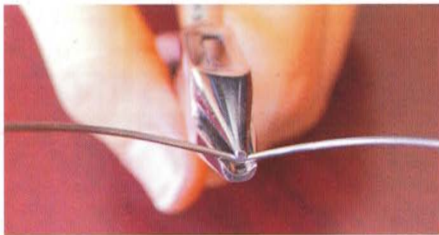
Fig. 105. Wire bending with the hollow chop plier in the middle of the wire.
