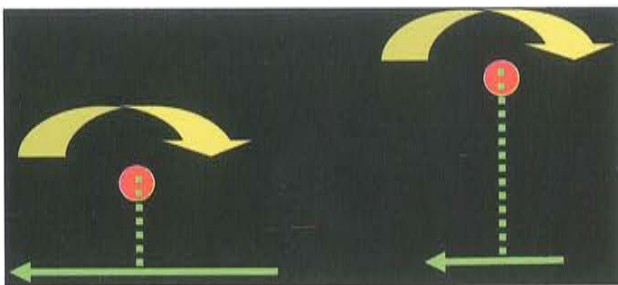
Fig. 11. Independently that the force magnitude is doubled and the distance to the center of resistance be reduced by half, or that the distance is duplicated and the magnitude of the force diminished, there will always be a tendency to produce rotation.
