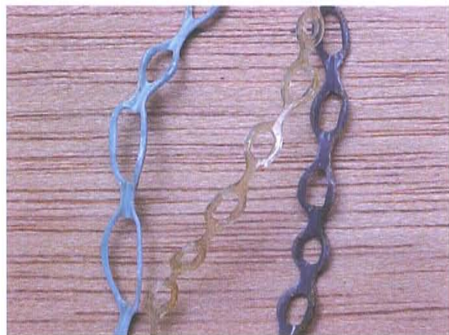
Fig. 1. Stained and deformed chains after 30 days use.
