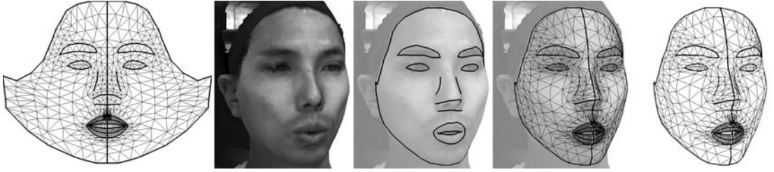
Figure 17.2 An example of a generic mesh (left) and its adaptation to 3D raw data based on feature lines. After the adaptation, specific regions can be extracted for further analysis.
