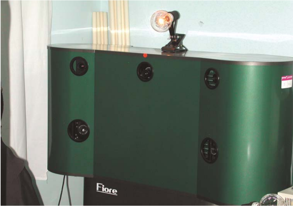
Figure 16.1 The Fiore 3D digitizer with two digital CCD cameras (top) and two light projectors (bottom).
