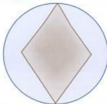
Fig. 8.12: Rhombus cross section of K-flex File
