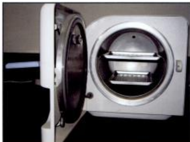
Fig. 7.2: Autoclave for moist heat sterilization
