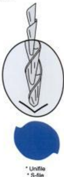
Fig. 8.17: Cross section and longitudinal shape of S-file
