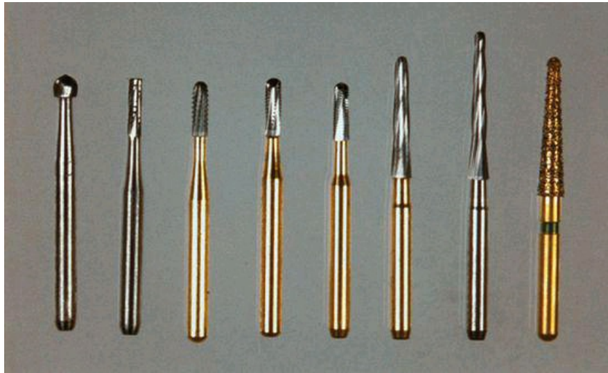
Figure 14-8 Examples of access burs. Left to right , No. 4 round carbide, No. 557 carbide, Great White, Beaver bur, Transmetal, Multipurpose bur, Endo Z bur, and Endo Access bur.
