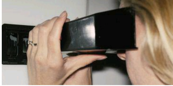
Figure 11-30 Magnifier-viewer blocks out peripheral light for better contrast. Contained within is a lens that magnifies the image four times.
