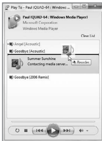
Figure 11-49: The PlayTo window provides simple playlist management features, including the ability to drag and drop content in from Windows Media Player.
