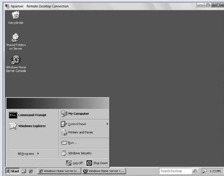
Figure 10-3: If you remotely access the server, you'll find a stripped-down version of Microsoft's enterprise-oriented Windows Server products.
