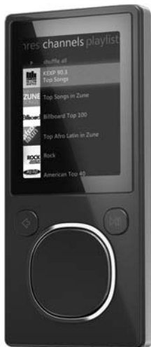
Figure 14-39: The Zune 8 and Zune 16 utilize flash storage and offer a small form factor.
