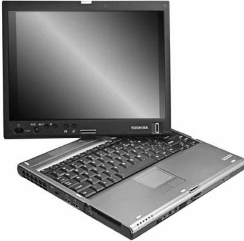
Figure 18-2: Convertible Tablet PCs have proven to be the most popular design because they can be used like a normal notebook computer when needed.
