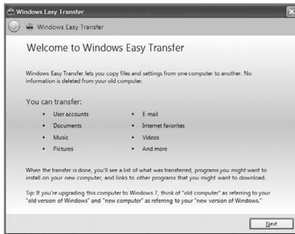
Figure 2-23: Windows Easy Transfer runs on your XP machine to back up important data before you install Windows 7.
