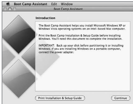
Figure 2-49: Boot Camp helps you configure a dual boot between Windows and Mac OS X.
