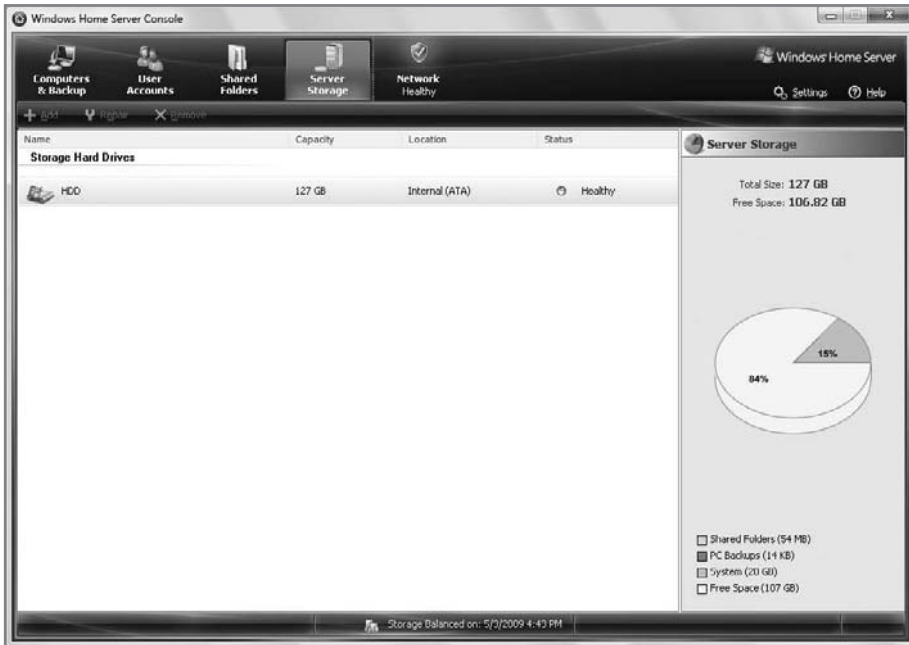
Figure 10-12: Server Storage shows which drives are configured for use with the server and how storage is allocated.
