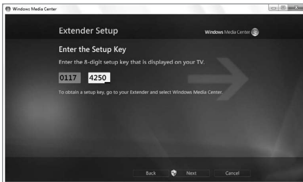
Figure 15-45: The Setup Key links an Extender to a single Media Center PC.
