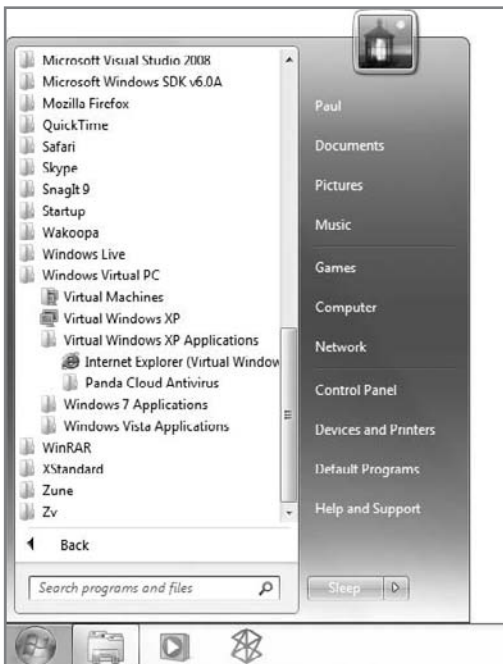
Figure 3-21: When you install applications in the virtual Windows XP environment, they also appear in the Windows 7 Start menu, so you can run them from there.
