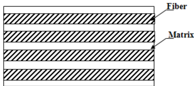
Fig. 1.1 Structure of a fibrous composite
