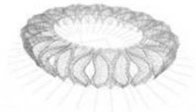
6. Secondary structural elements for truss tracing and roof systems are linked to the primary truss system.
