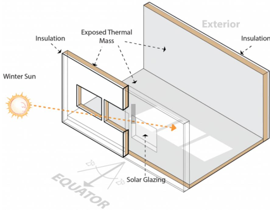
The surface area of concrete exposed to over the day is 9 times the area of the solar glazing. The illustrations represent a space with glazed openings and masonry walls and floor. The walls are a light color and the floor a medium color.
