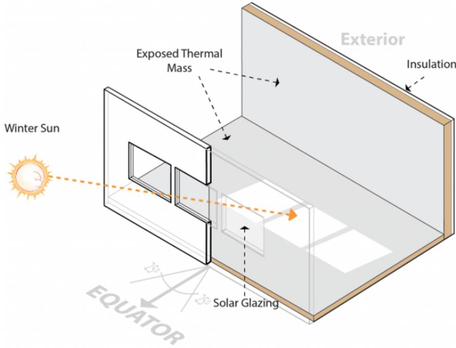
The surface area of concrete exposed to over the day is 3 times the area of the solar glazing. The illustrations represent a space with glazed openings and light colored interior surfaces and a medium colored thermal mass floor or wall.
