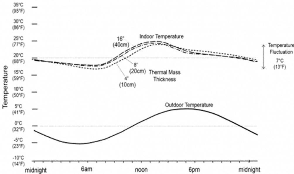
The graph illustrates space air temperatures for a glazing area to thermal mass surface area ratio of 9:1 and mass thicknesses of 10, 20 and 40 centimeters (4, 8 and 16 inches). An increase in masonry thickness beyond 10 centimeters (4 inches) results in little change in space temperature fluctuation. The temperature fluctuation over the day is approximately 7°C (13°F).
