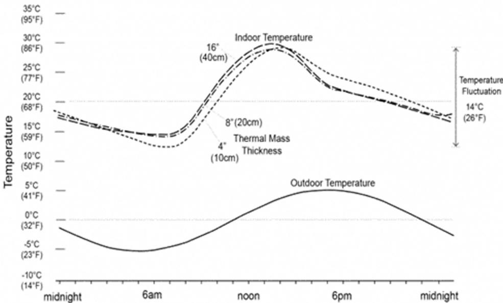
The graph illustrates space air temperatures for a glazing area to thermal mass surface area ratio of 3:1 and mass thicknesses of 10, 20 and 40 centimeters (4, 8 and 16 inches). An increase in masonry thickness beyond 20 centimeters (8 inches) results in little change in space temperature fluctuation. The temperature fluctuation over the day is approximately 14°C (26°F).
