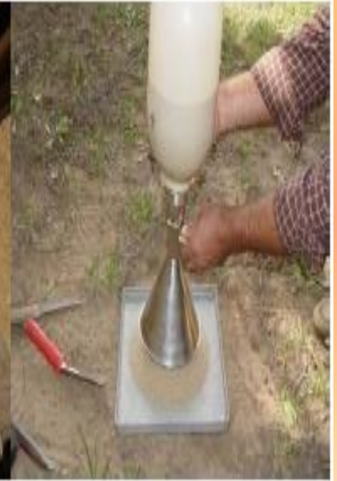
Sand cone test
