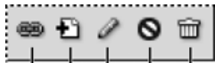
A B C D E A. Attach Style Sheet B. New CSS Rule C. Edit Style D. Disable/enable CSS property E. Delete CSS rule
