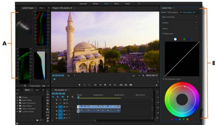
A Lumetri Scopes panel B Lumetri Color panel with curves, color wheels, and slider adjustments
