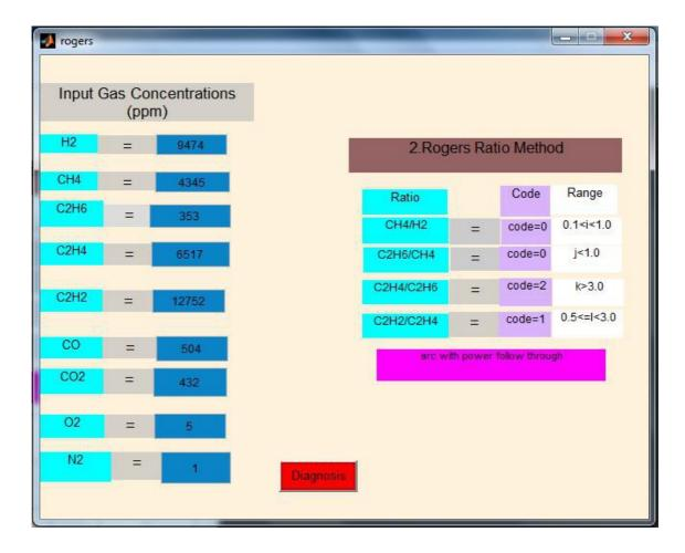
Figure 6.1 Result window of Rogers Ratio Method using MATLAB GUI
