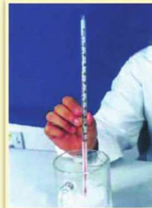
The measuring temperature of liquid is used by Celsius thermometer
