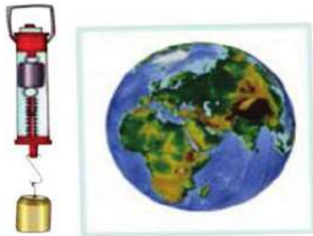
Fig (1-13): The object's weight on the Earth's surface is equal to 6 Newton.
