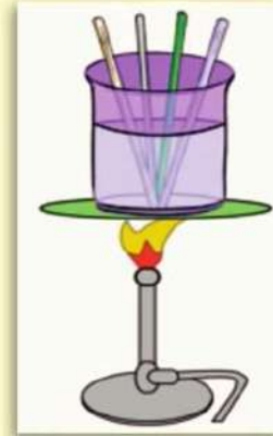
Fig (2-2) The difference in materials leads to the difference in conducting heat.
