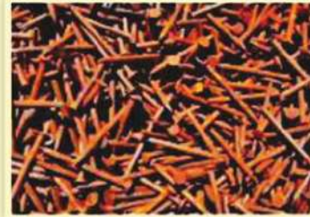
Fig (3-10) Rusty nails after exposure to moisture
