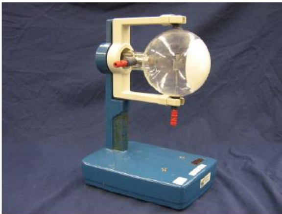
Figure 1: Maltese Cross Tube.
