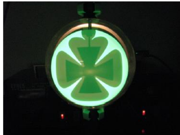
Figure 2: Deflected Electron Shadow.
