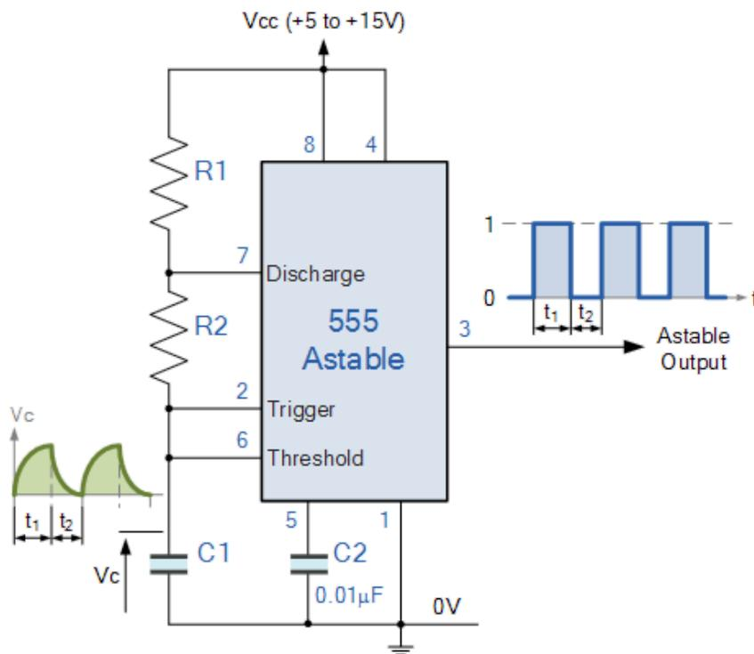
$$T_1 = 0.7(R_1 + R_2)C$$
