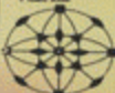
Cubic (Isometric) 1 mirror of symmetry 9 mirror planes 3 twofold axes 4 threefold axes 3 dead axes
