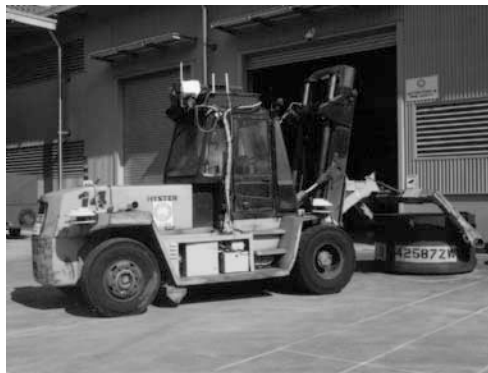
Figure 1: A Hot Metal Carrier picking up the crucible.
