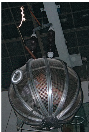
FIGURE 2.32 A person inside a Faraday cage is unharmed by a large voltage applied outside the cage, which produces a huge spark. This demonstration is performed several times daily at the Deutsches Museum in Munich, Germany.
