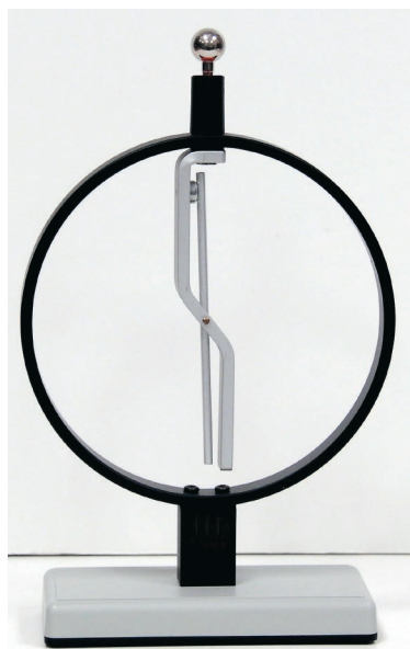
FIGURE 1.8 A typical electrostatic demonstration electroroscope used in lecture demonstrations.
