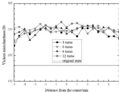
Figure 1. The average Vickers microhardness, Hv, versus distance from the center of the disks of original state of 7085 Al alloy and processed by HPT after various turns under pressure of 2 GPa.
