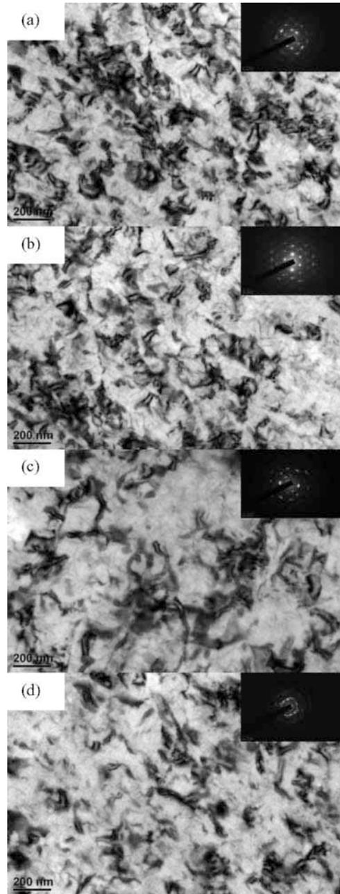
Figure 4. TEM micrographs and SAED patterns of Al 7085 alloy
