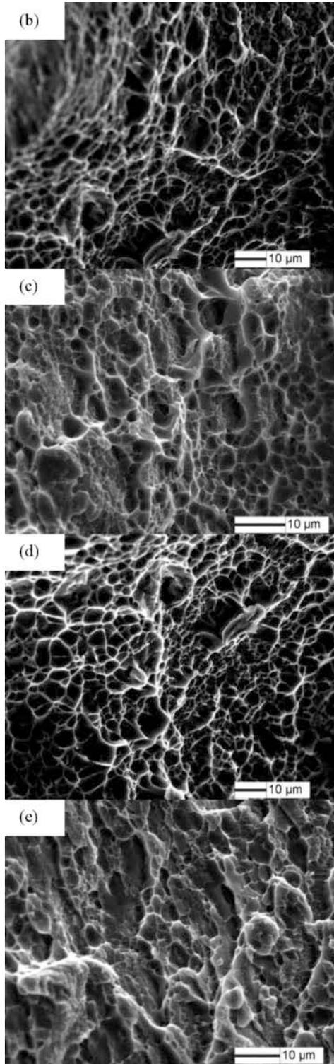
Figure 3. SEM fractographs after tensile test of disks processed by HPT through 3 turns (a), 6 turns (b), 9 turns (c), 12 turns (d) under pressure of 2 GPa and disk in original state (e).
