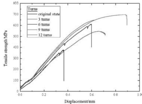
Figure 2. Tensile strength versus displacement curves of tensile tests for original state sample and disks processed by HPT after various turns under pressure of 2 GPa.
