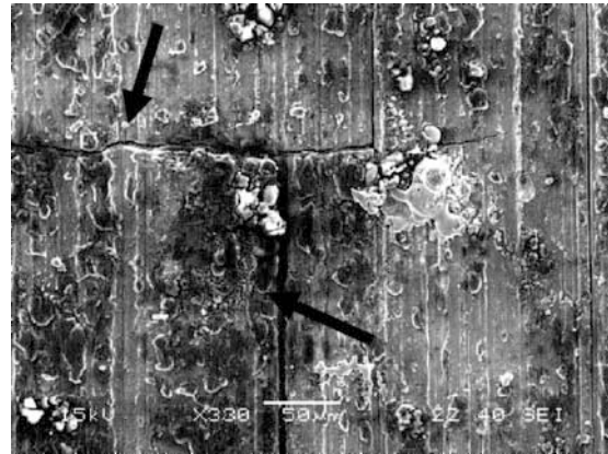
Figure 2. Longitudinal and transverse cracks on the shell surface.
