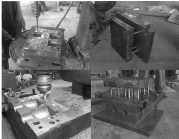
Figure 19: Drilling, Milling, Ejection system assembly and Assembled die blocks
