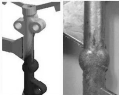
Figure 5. Validation of simulation result with the real casting. From simulation liquid metal from ingate2 (yellow) merge with that of ingate1 (blue) at the middle of the part.
