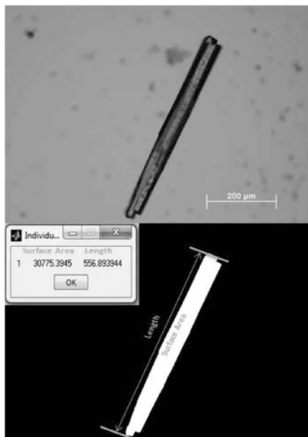
Figure 1 Principle of UQ Hydrometallurgy Image Analysis software
