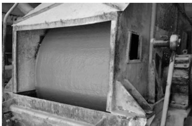
Figure 9. Filtration of thickener underflow
