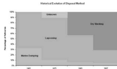
Figure 1.2 - Evolution of storage practices at 17 refineries currently in operation (CSIRO)
