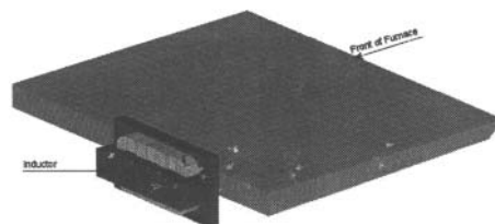
Fig 6 showing the location and preparation of the cfd grid ready for modeling the stirrer on a side mounted application.
