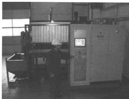
Figure 1. Length wise graphitization furnace for Ø50mm cores
