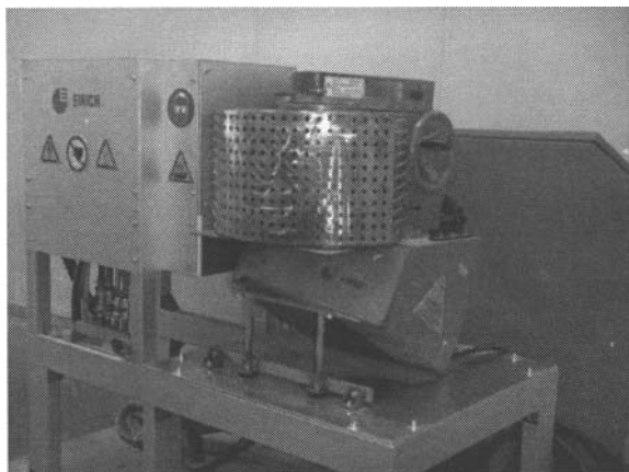
Figure 2: Mixer with inductive heating
