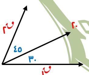
$$R_{H_1} = \frac{20 \times \cos 45^\circ}{\cos(45^\circ + 30^\circ)} = \frac{20 \times \cos 45^\circ}{\cos 75^\circ} = 14.7 \text{ نيوتن}$$
