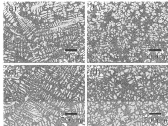
Figure 6. Microstructures which correspond to the cooling curves shown in Fig. 5. The end temperatures of the vibrations were; (a) no vibration, (b) 863 K, (c) 892 K, (d) 888 K.
