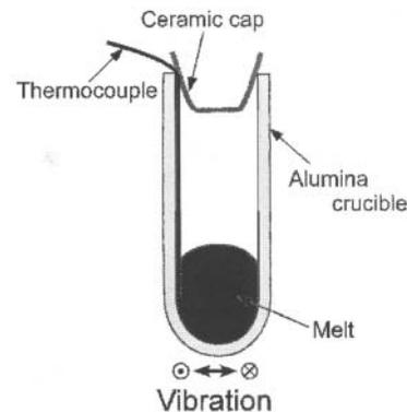
Figure 1. Schematic illustration of the alumina crucible where the molten specimen was put in.
