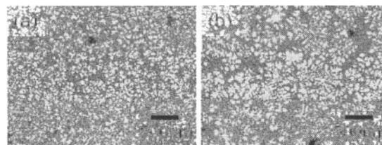
Figure 4. Microstructures in the specimens solidified during imposition of the mechanical vibrations (50 Hz, 702 mm/s); (a): in the alumina crucible shown in Fig. 1; (b): in the alumina crucible shown in Fig. 3.
