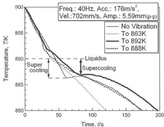
Figure 5. Cooling curves for the specimens solidified during imposition of the mechanical vibrations (40 Hz, 702 mm/s). The end temperature of the mechanical vibrations was varied.
