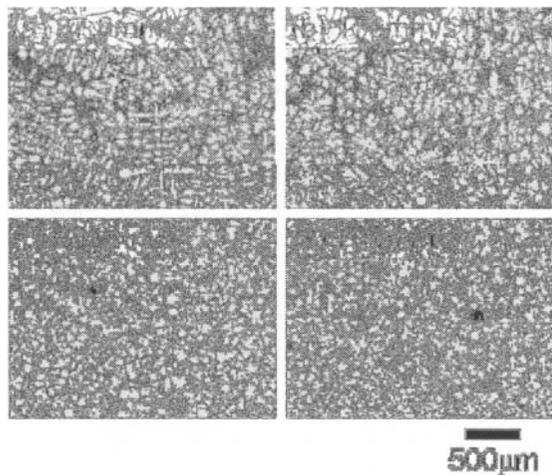
Figure 2. Microstructures in the specimens solidified during imposition of the vibrations with same frequency 50 Hz.
