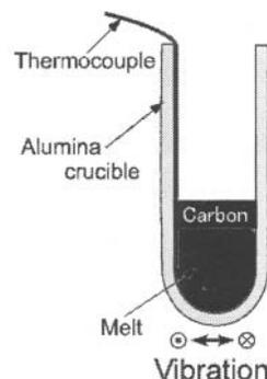
Figure 3. Schematic illustration of the alumina crucible. The melt is locked by a carbon block which was fixed to the crucible.
